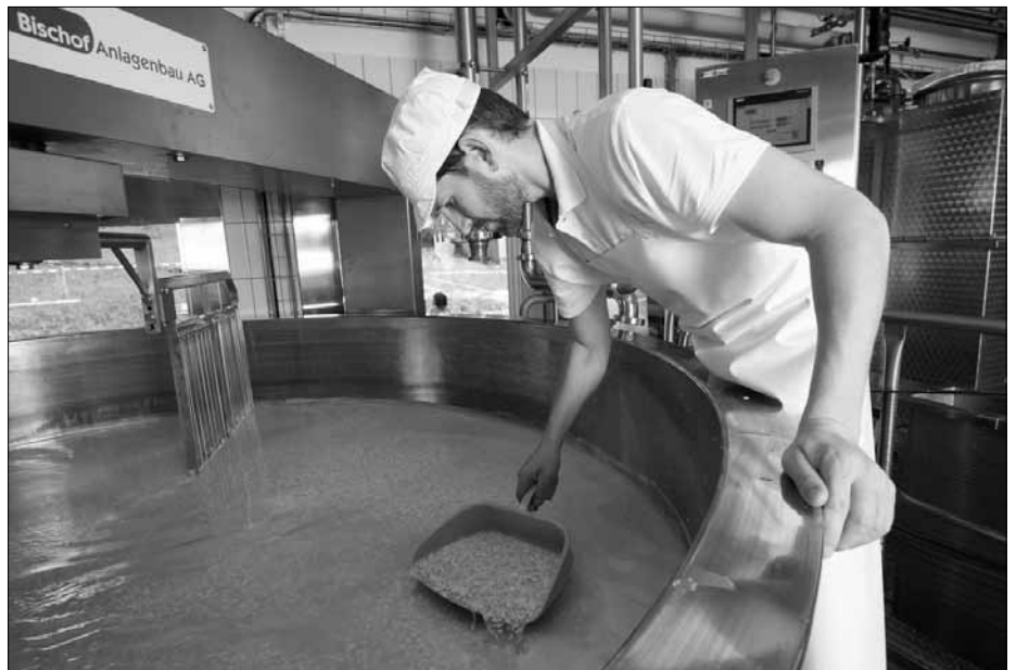
After the curd is cut with harp, the cheese granulation is being checked. (picture Alpkäserei Urnerboden)
