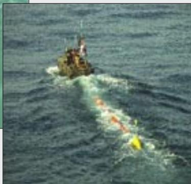
To speed up operations, the RN had leased the German Sea Fox Mine Disposal System, which was optimised for operations in strong tidal streams and poor visibility, and a remote-controlled Shallow Water Influence Mine Sweep System.
