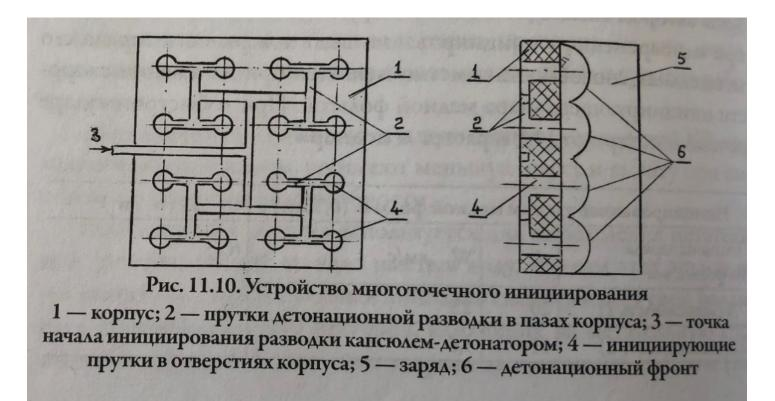
Figure 4. Danilenko's schematic of a multi-point detonation system.
