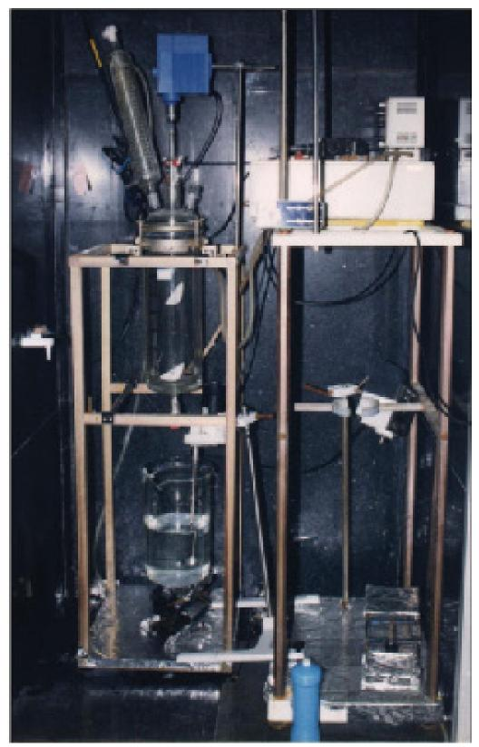
Figure 15. Recrystallization reactor image from the archive.
