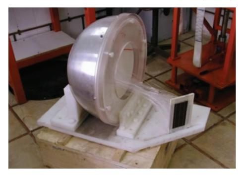
**Figure 8.** Model of an experimental system in the Nuclear Archive representing what appears to be a shock wave generator and high explosive, with a diagnostic system using fiber optic cables, to measure time of arrival of a detonation front in the main charge.
