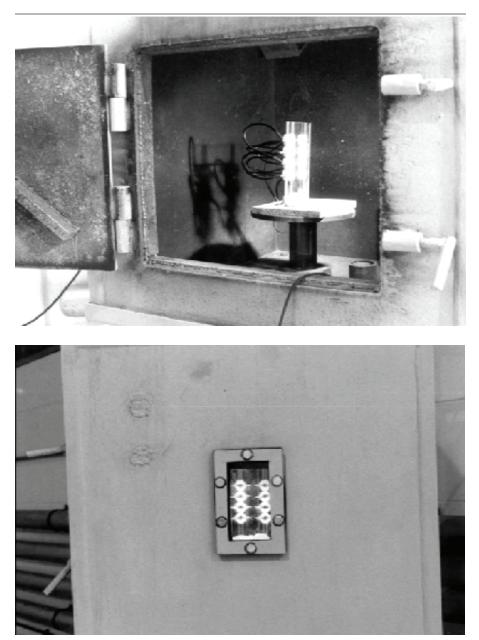
Figure 20. Two photographs from the archive of the Lower-Nour Abad blast chamber with eight EBWs or detonators visible.
