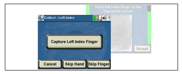
With the fingerprint capture screen active, have the subject put a fingerprint on the fingerprint sensor, located on top of the HIIDE. The preview window displays the fingerprint. To complete enrollment of that finger press the "Accept" button, or one of the shoulder triggers.
