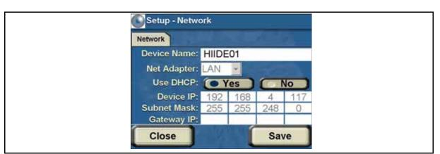
Figure 60. Setup - Network screen
