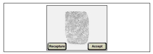
If the image meets enrollment standards the "Accept" button will save the image, and the next collect screen will be displayed. If the image does not meet enrollment standards the "Recapture" button will return the fingerprint capture process back to Step 1: Have the Subject Place Finger on the Sensor.
