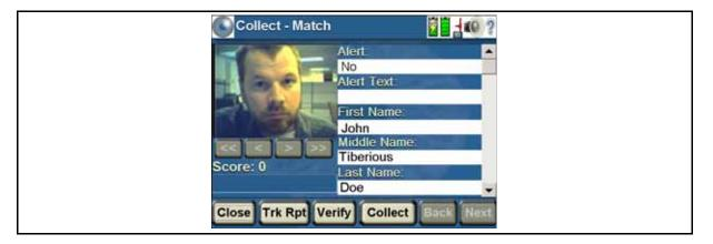
The Collect - Match screen displays the biographical data of the matched individuals. Use the scroll bar to view all information about this subject. If a face image is in the database it will also appear as displayed in Figure 14. If additional images are available in the match, the buttons below the image will become active. The buttons at the bottom of the Collect - Match screen are described below.
